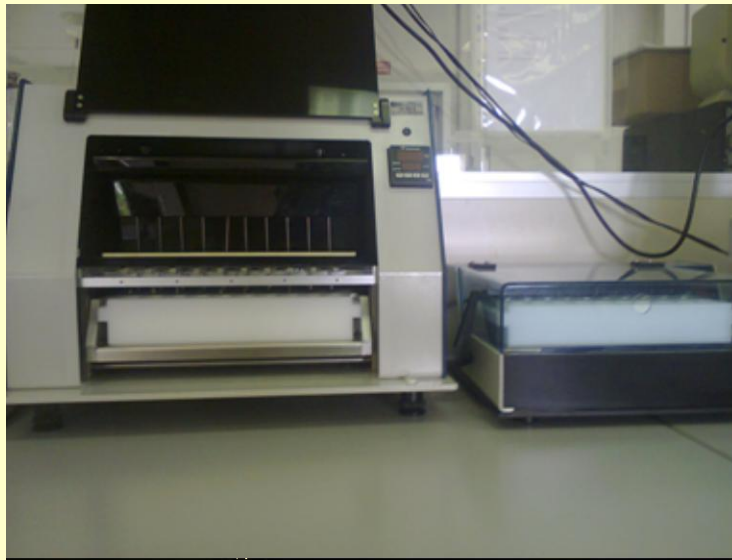
Fomagraph instrument for lactodynamographic analysis
