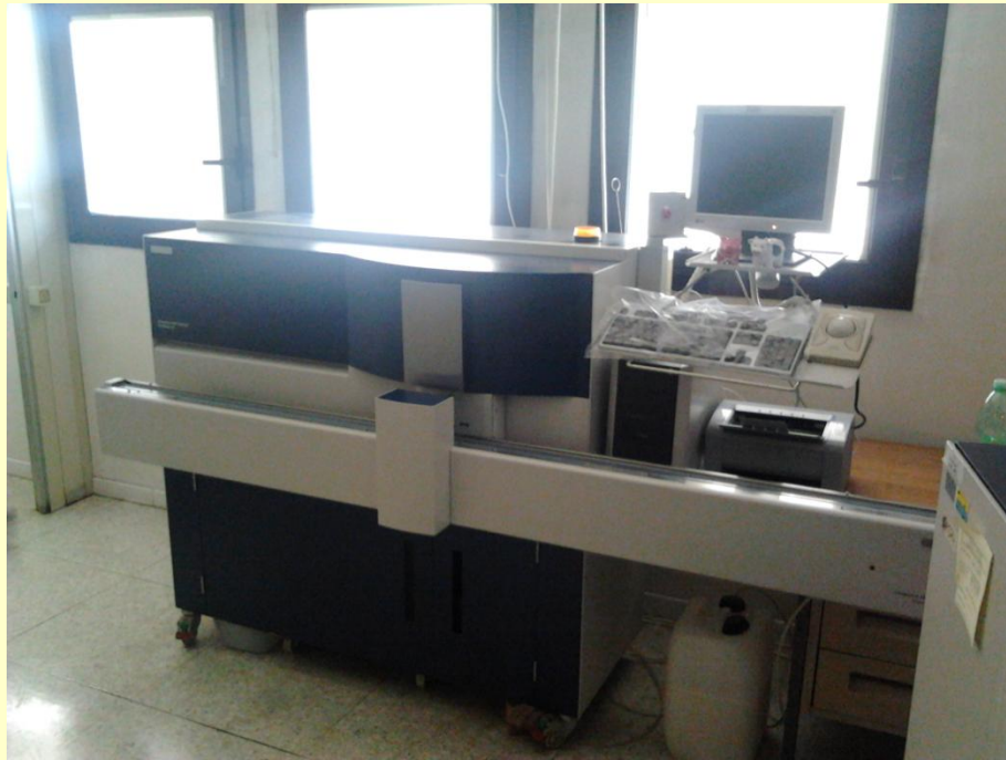
Bactoscan FC apparatus for TBC analysis
